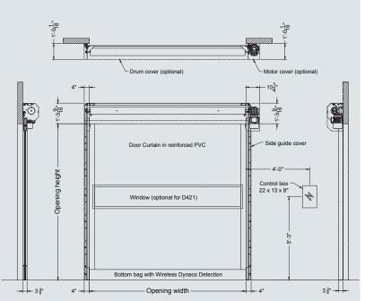
All indicated dimensions are net: the space necessary for mounting and maintenance has to be provided.
