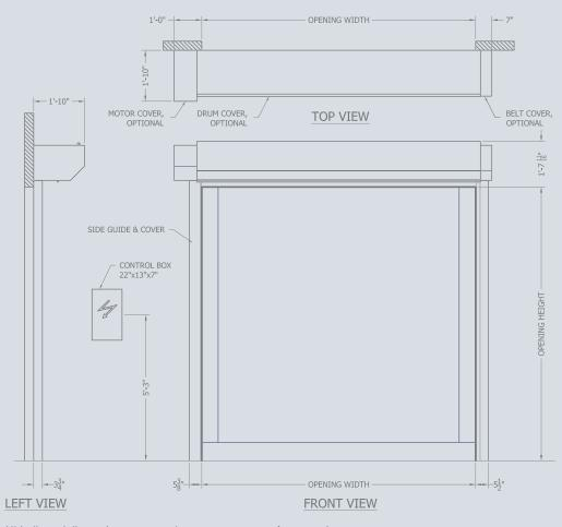
All indicated dimensions are net: the space necessary for mounting and maintenance has to be provided. REMARK: based on the risk analysis of the environment, extra push buttons, detectors and covers might be required.
